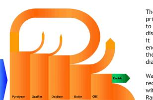
The Pyroclast is primarily designed to address waste disposal. However, it may also produce energy, as shown in the adjacent Sankey diagram.
