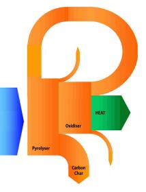
The Pyroclast is primarily designed to address waste disposal. However, it may also produce energy, as shown in the adjacent Sankey diagram.
